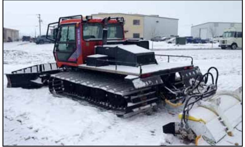
THIS IS THE MACHINE THAT WILL BE GROOMING OUR TRAILS NEXT SEASON. IT WILL HAVE 2 TRACK-SETTERS ATTACHED BEFORE DELIVERY TO LOST TRAIL.
